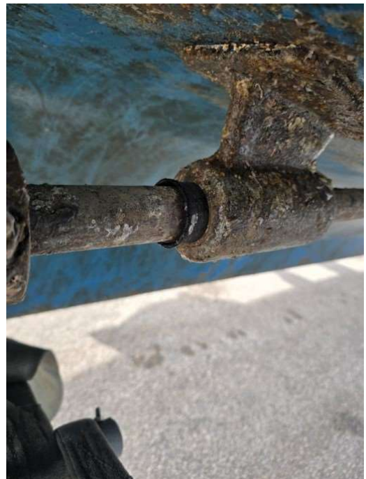
Cutlass bearing material loose and sliding out from inside strut
